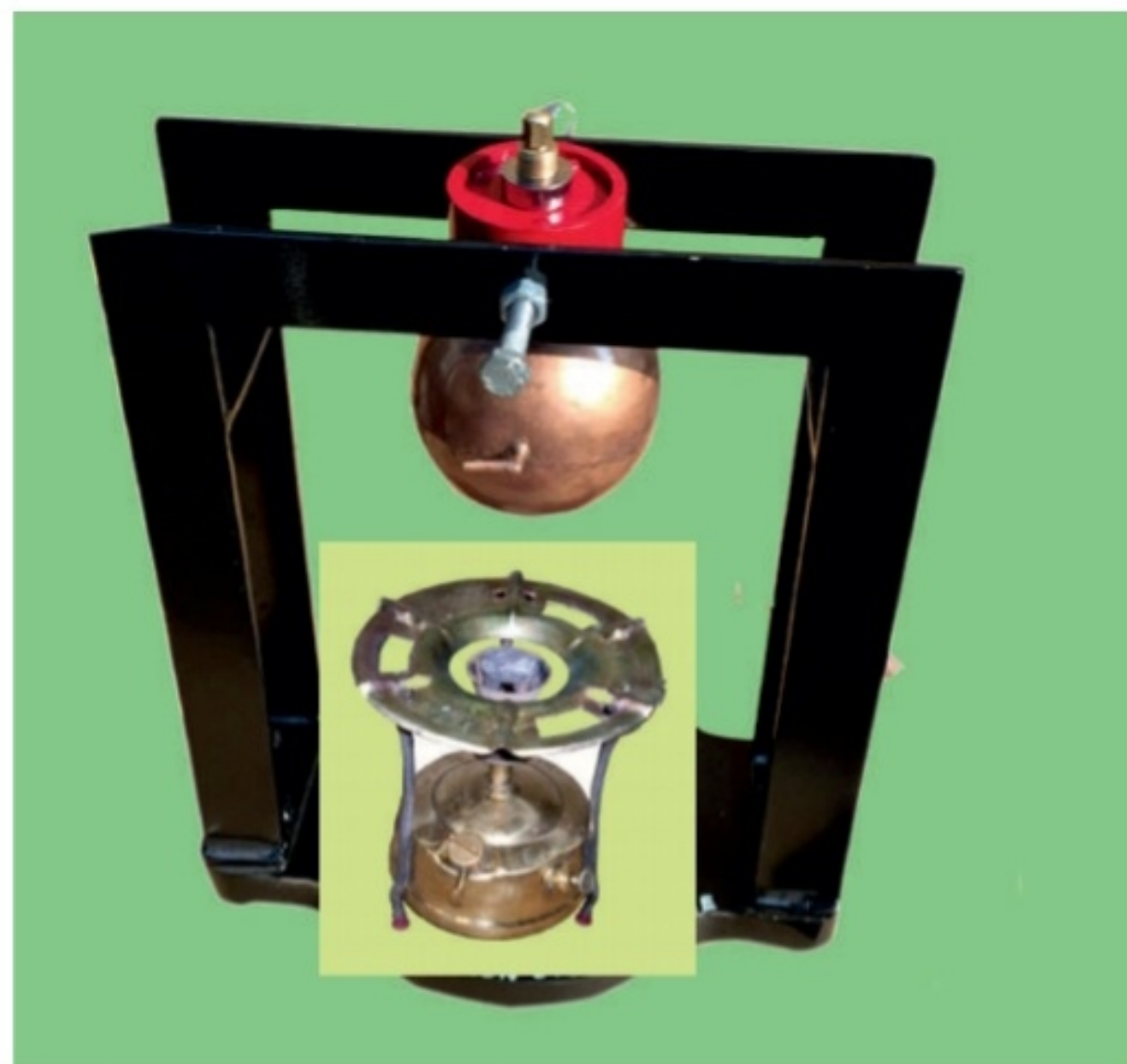
HERO'S STEAM REACTION TURBINE
